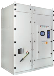
Spain Soft-starter for 3300V, 250A with incoming compartment, disconnect switch and a fuse base.
